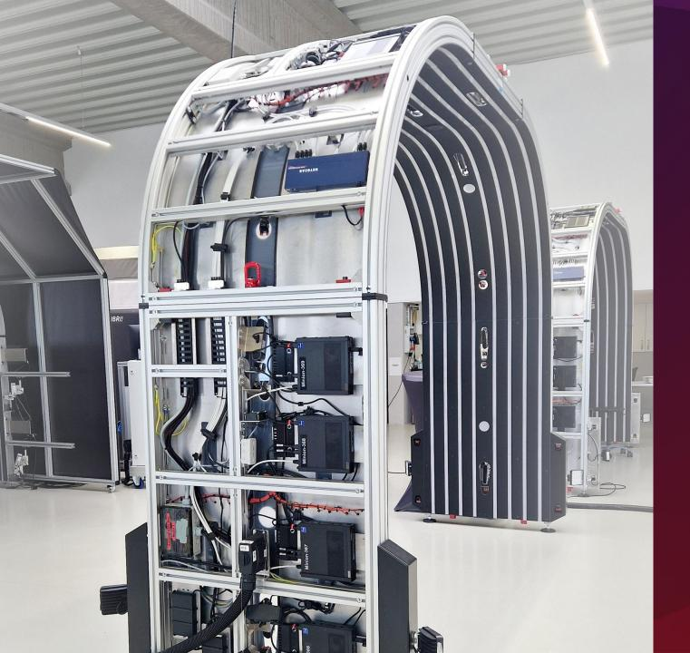
Each Colibri scanner takes advantage of the performance of a Lenovo ThinkStation P3 Tiny workstation to process huge volumes of data streaming from 2D and 3D high-resolution cameras.
